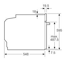
measurements in mm
